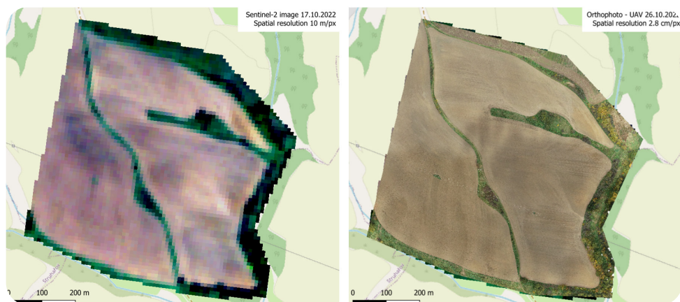
Fig. 4: Comparison of Sentinel-2 true-colour satellite image with 10 m/pixel resolution and orthophoto map taken by UAV with 2.8 cm/pixel resolution with visible erosion furrows, which can also be used for more detailed analysis, e.g. calculation of eroded material.
