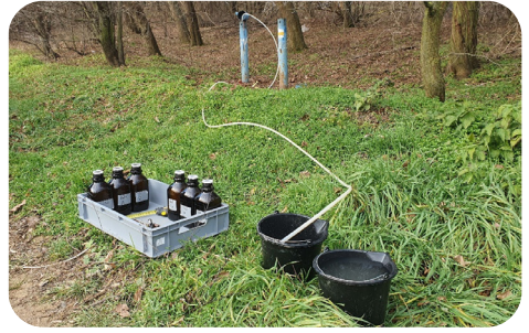
Fig. 2: Sampling of shallow subsurface water for nitrate monitoring.
