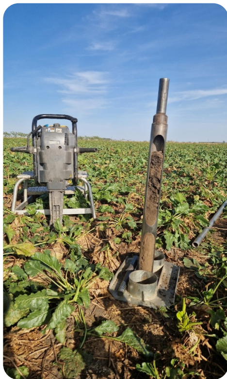
Fig. 1: Drilled, undisturbed soil sampling to identify the nitrate profile under an arable parcel.
